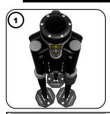
Stand the tripod up with the base plates on the ground and release the Velcro Strap.
