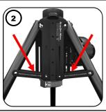
Unfold the tripod legs and make sure the cross bars are locked into position.
