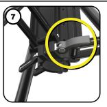
Release the cam lock on the bottom of the tripod.
