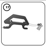
Unwind the rope while walking away from the mast. Take one normal step for each meter of height of the mast. Stop, unwind the remaining guy rope and drive a stake into the ground. Then attach the guy rope.
