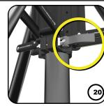
Holding the center mast pole, slowly release the cam lock.
