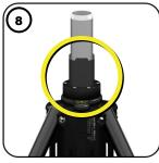
Insert first mast pole leaving at least 4 Inches above the tripod collar
